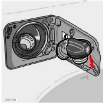
The fuel filler cap can be placed on the hook on the fuel filler door while refueling
