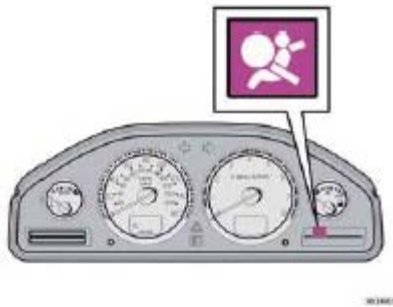
SRS warning light
