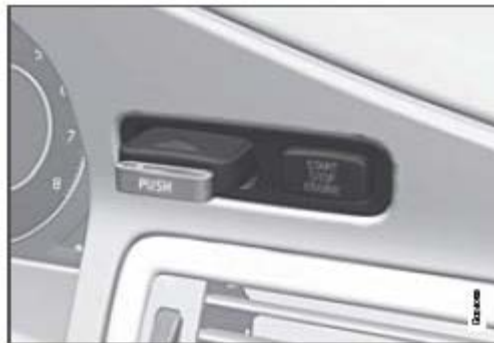
Ignition slot with remote key, start/stop button
