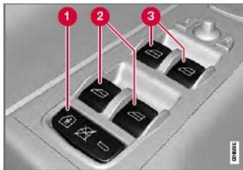
Driver's door control panel
