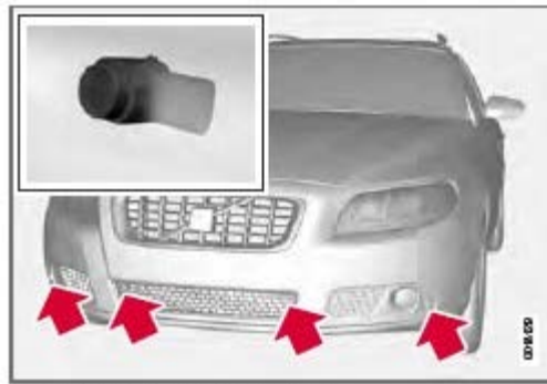
Location of the front sensors
