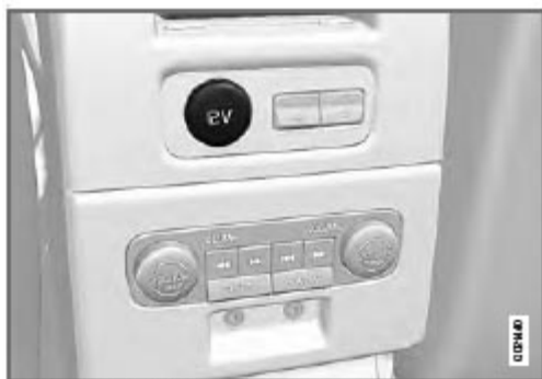
12-volt socket in the rear center console
