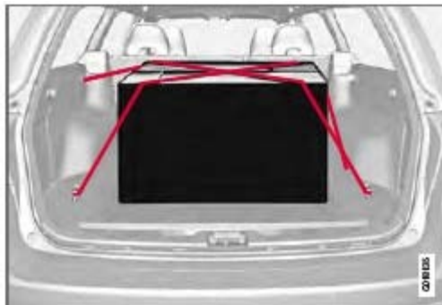
Load secured in upper and lower hooks
