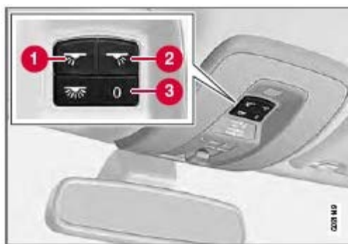
Light switches, front roof lighting
