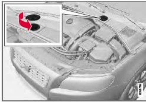
Location of the brake fluid reservoir
