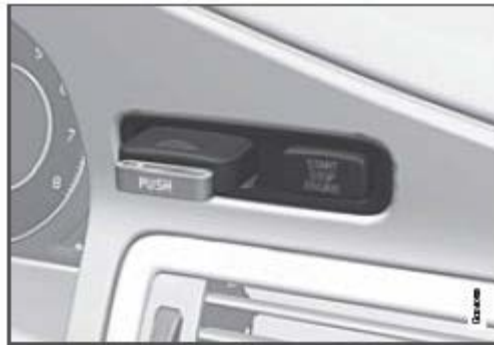
Ignition switch with remote key inserted (see page 80 for more information)
