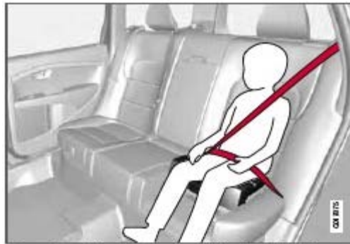
Correct seating position: child's head is below the head restraint and the shoulder belt is across the collarbone
