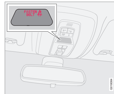
Seat belt reminder light in ceiling console
