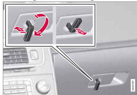
Locking/unlocking points with valet locking activated
