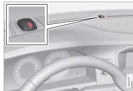
Lock/alarm indicator light
