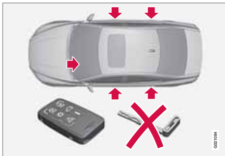
Locking/unlocking points with valet locking activated
