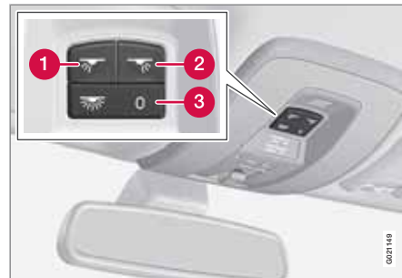
Light switches, front roof lighting
