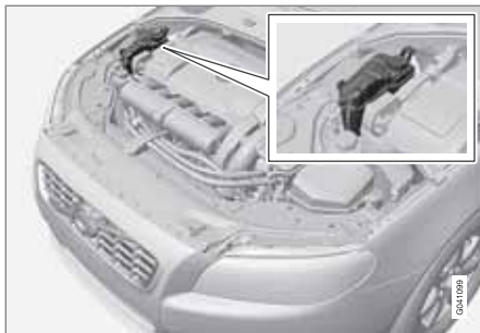
Location of the coolant reservoir
