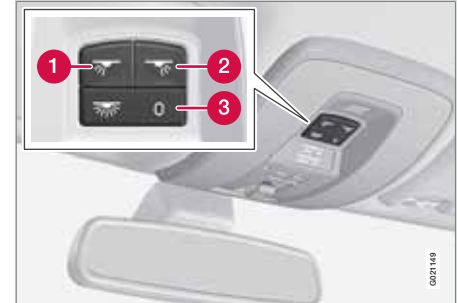
Light switches, front roof lighting
