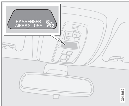
Occupant Weight Sensor (OWS) indicator light
