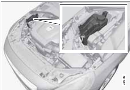
Location of the coolant reservoir
