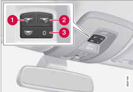
Light switches, front roof lighting
