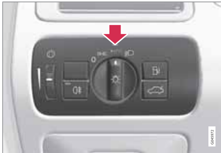
Light switch in the AUTO position
