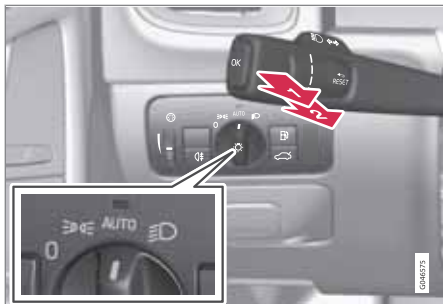
Headlight switch with AUTO and lever
