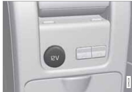
12 V socket in tunnel console, rear seat.
