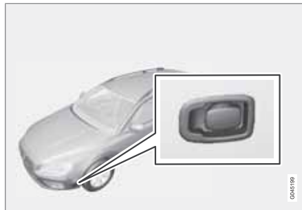
Electrical input to the engine block heater.
