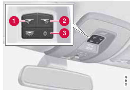
Light switches, front roof lighting
