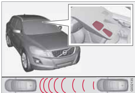
Location of the laser sensor in the windshield 2
