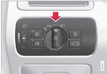
Light switch in the AUTO position
