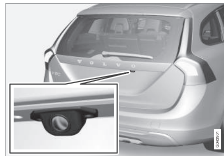
Camera location next to the opening handle.
